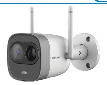
KN-2003WN.PIR delivers 2MP live monitoring, it supports the latest H.265 compression which can save up to 50% bandwidth and storage. With IP67 certified, the camera can be used outdoors under different weather conditions. With built-in spotlight and 110dB security siren, KN-2003WN.PIR actively keeps unwelcome visitors away from what you care about.
