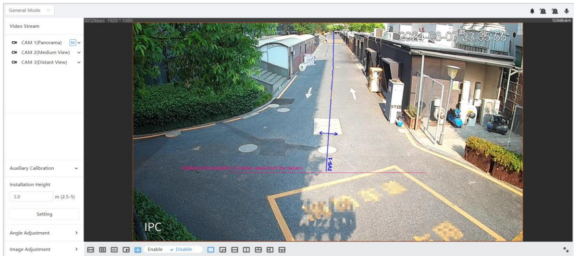
Figure 7-7 Configure auxiliary calibration
